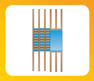
This is manufactured similar to L fin except that the base tube is knurled before wrapping the 'L' shaped fin strip. After wrapping the fin strip, the fin foot is pressed over the tube knurl & tension wound on the base tube to increase the bonding between the tube & fin. This will result in increased heat transfer performance.
