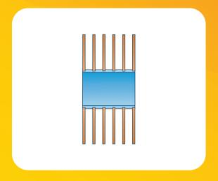
Aluminium fin strip is wound & embedded on a groove and securely locked by closing the groove with the base tube metal. This ensures maximum heat transfer at high temperatures.
