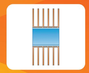
Aluminium fin strip is formed to LL shape and tension wound on the tube with overlapping of fins as shown in the figure.
