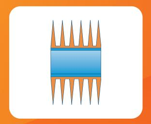
The finned tubes for construction of heat exchangers for the range of temperatures from 233° to 598° K (-40° to 325°C). The fin OD ranging from 38 mm to 82.55mm.
