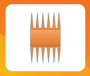
This is similar to the extruded Bimetallic. Except that there is no inner base tube. The tube & fins are made out of the single aluminium tube.
