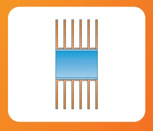
Aluminium fin strip is formed to L shape and then tension wound to the base tube.
